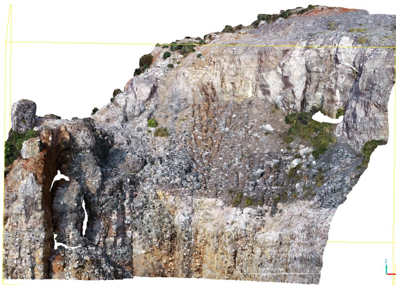
Figure 16. Point cloud data after edge segmentation
