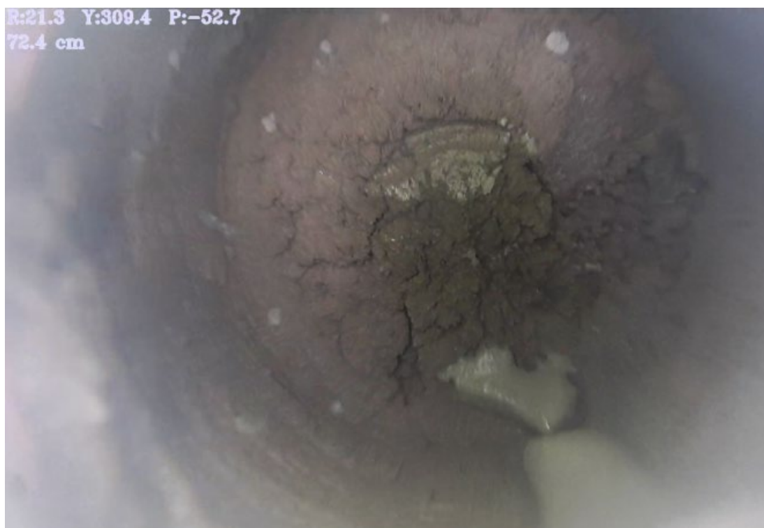
Figure 10. Screenshot from borehole video of ZK2 (outside the air-gap anomaly zone)
