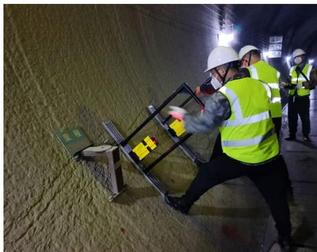
**Figure 5.** Site photo of geological radar survey work
