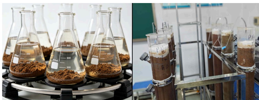
Figure 1. Left: Laboratory batch leaching experiment; Right: Laboratory column leaching experiment
