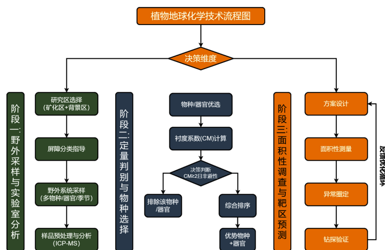
Figure 5. Plant geochemical technology flow chart
