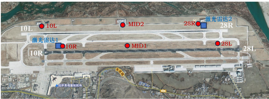
Figure 1. Locations of wind measurement equipment at Lhasa Gongga International Airport. The red dots represent the auto-matic surface weather observation system, and the blue squares represent the Molas 3D wind lidar 图 1. 拉萨贡嘎国际机场的测风设备部署位置。红色圆点为地面自动气象观测系统，蓝色方块为 Molas 3D 测风激光雷达
