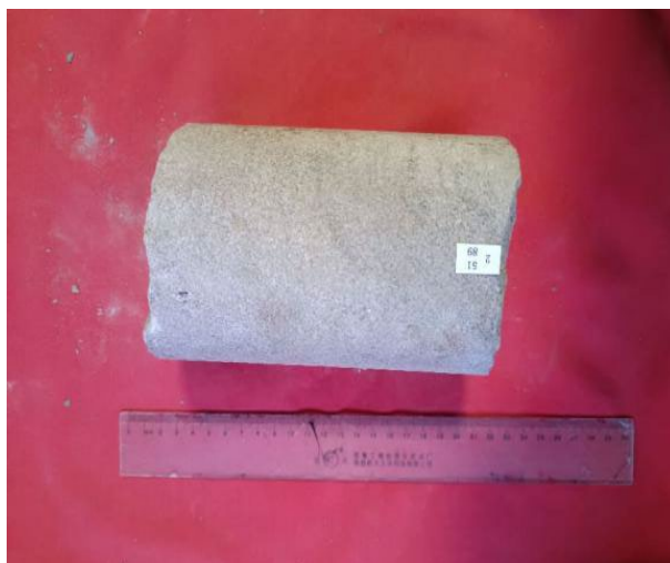
Figure 4. Sedimentary structure characteristics of the Sha-1 Member (gray siltstone with tabular cross-bedding at 1910.12 m)
