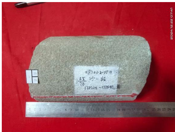
Figure 3. Sedimentary structure characteristics of the Sha-1 Member (grayish-green fine sandstone with horizontal bedding at 1735.24 m) 图 3. 沙一段沉积构造特征(灰绿色细砂岩 水平层理 1735.24 m)
