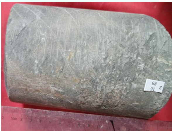
Figure 2. The rock color characteristics of the Sha-1 Member in the study area (gray argillaceous siltstone at 1902.6 m) 图 2. 研究区沙一段岩石颜色特征(灰色泥质粉砂岩 1902.6 m)
