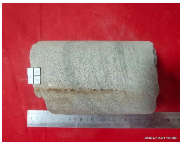
Figure 5. Sedimentary structure characteristics of the Sha-1 Member (grayish-green fine sandstone with trough cross-bedding at 1738.9 m)
