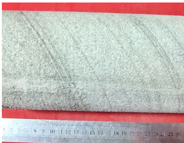
Figure 1. The rock color characteristics of the Sha-1 Member in the study area (light gray fine sandstone at 1758.6 m) 图 1. 研究区沙一段岩石颜色特征(浅灰色细砂岩 1758.6 m)
