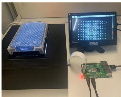
Figure 1. Image acquisition system based on Raspberry Pi 图1. 基于树莓派的图像采集系统
