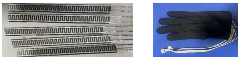
Figure 5. Membrane pressure sensor and teaching gloves 图 5. 薄膜压力传感器和示教手套
