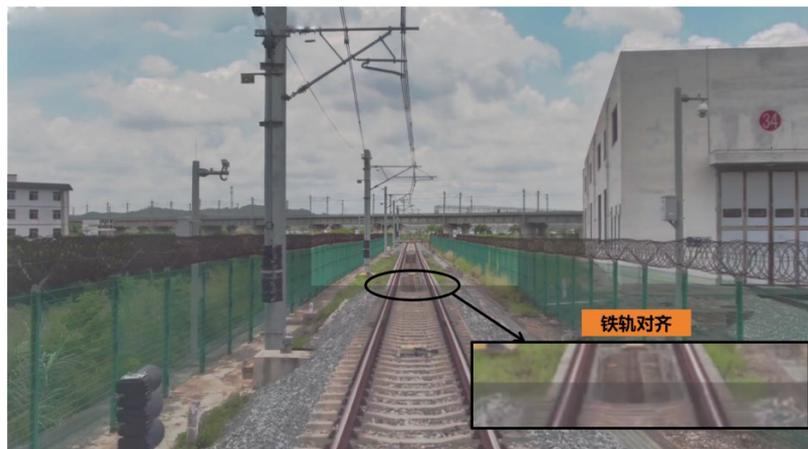
Figure 6. Fused image after fine registration using the phase correlation method
