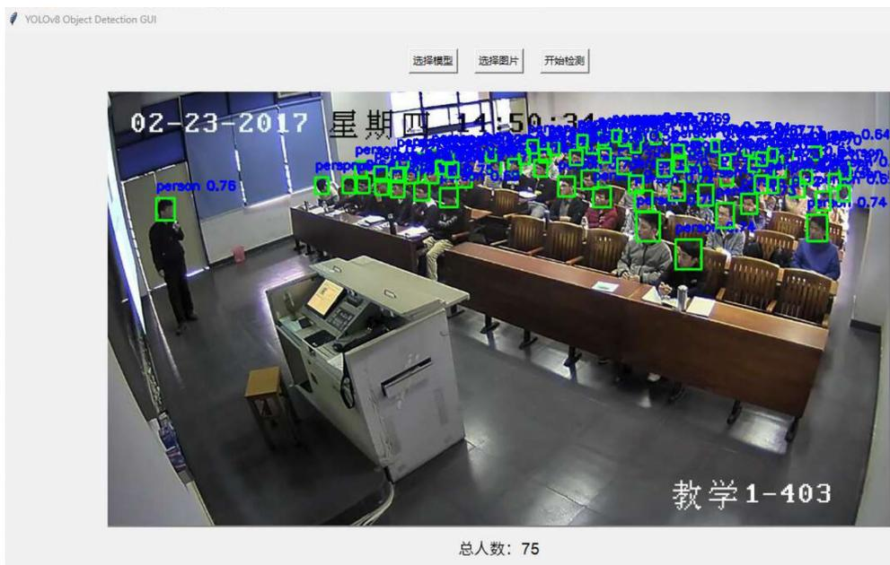
Figure 12. Schematic diagram of detection results in spacious classroom
