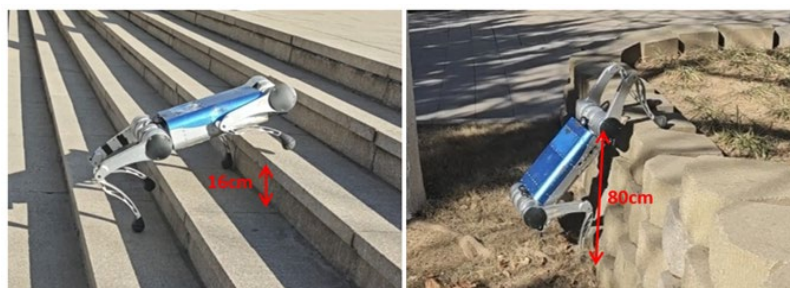
Figure 7. The Y15 robot climbing 16 cm high stairs and descending from an 80 cm platform
