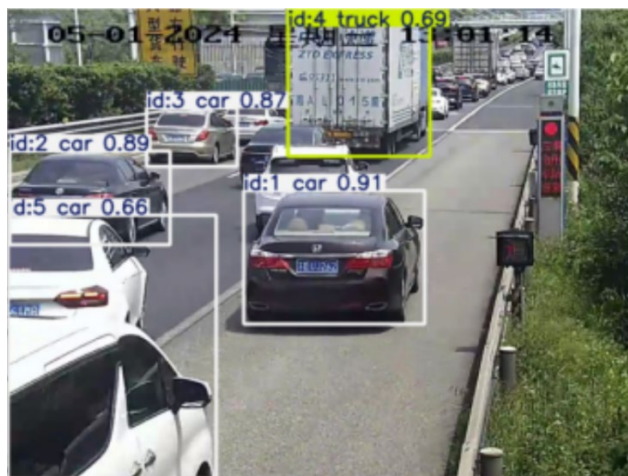
Figure 2. Schematic diagram of vehicle recognition and tracking
