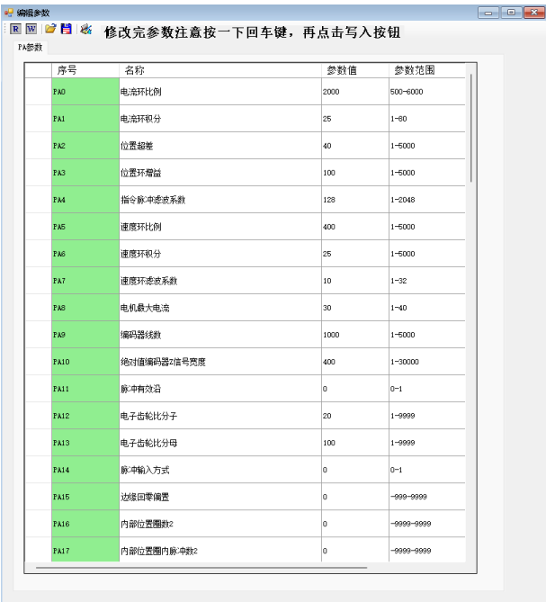
Figure 2. Schematic diagram of the driver settings interface in the valve control system 图 2. 阀门控制系统中驱动器设置界面示意图
