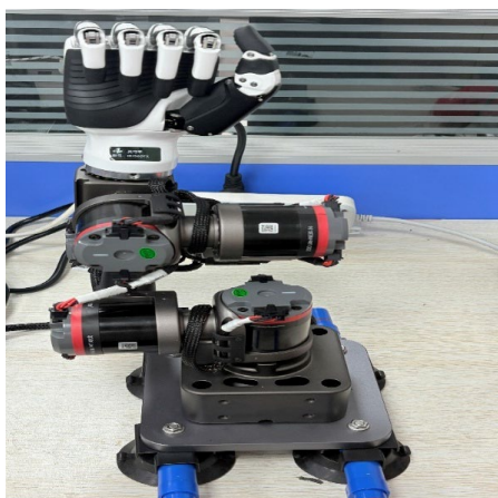
Figure 9. Robotic end-effector: the 6-DOF manipulator and five-fingered dexterous hand
