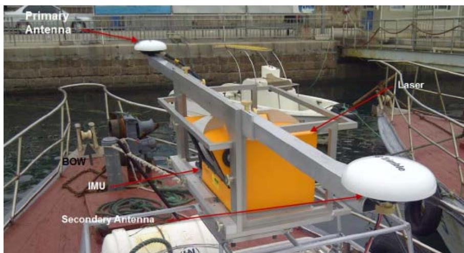
**Figure 2.** Installation diagram of laser scanner and inertial navigation and attitude measurement system
