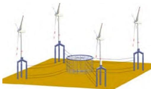
Figure 4. Offshore wind power foundation mooring—integrated development model of common structures 图 4. 风电基础系泊 - 共结构融合发展模式
