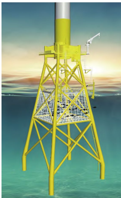
Figure 3. Co-use model of wind turbine units and aquaculture cage structures
