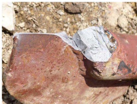
Figure 2. Saddle shaft fracture 图 2. 鞍座轴断裂
