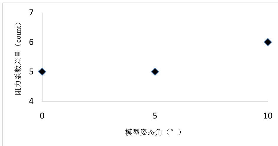
Figure 6. Difference of drag coefficient of standard model under different test conditions
