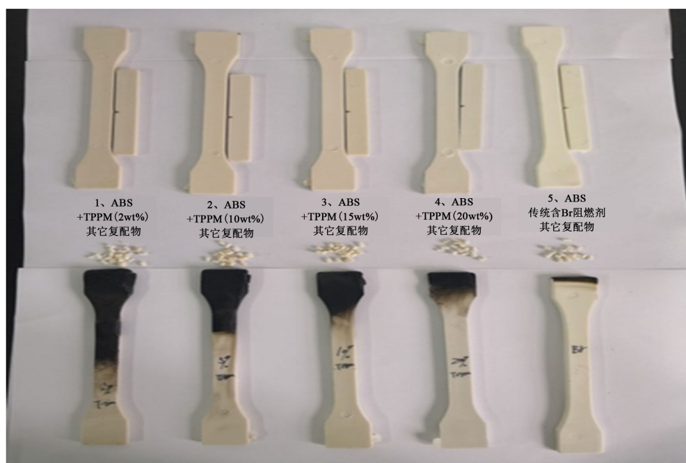
Figure 4. Flame retardant effect of samples containing TPPM
