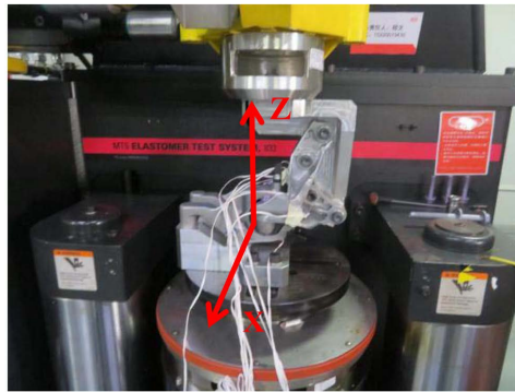
Figure 3. Drawing of the motor suspension measurement point 图 3. 电机悬置测点示意图
