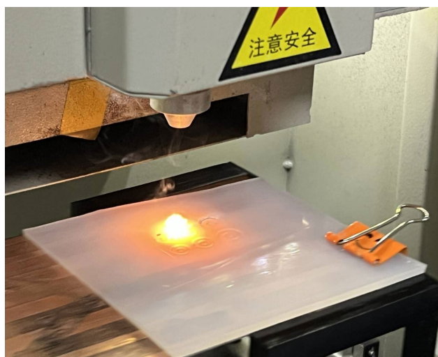
Figure 4. Schematic diagram of continuous laser pyrolysis processing technology
