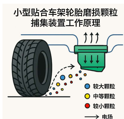
Figure 2. Working principle diagram of the compact frame-mounted tire wear particles collection device
