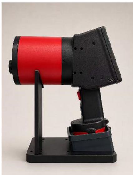
Figure 4. Emissivity measurement instrument photograph
