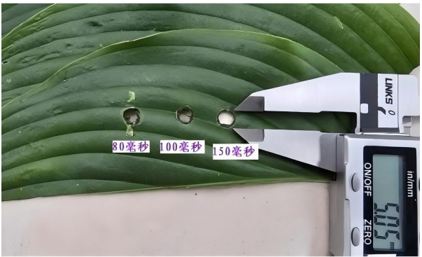
Figure 8. Measurement of output light spot of blue light module 图 8. 蓝光模块输出光斑测量
