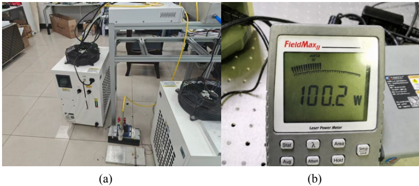
Figure 6. Blue light weeding experiment platform: (a) Weeding experiment platform; (b) Fiber output power of the blue light module 图 6. 蓝光除草实验平台: (a) 除草实验平台; (b) 蓝光模块光纤输出功率
