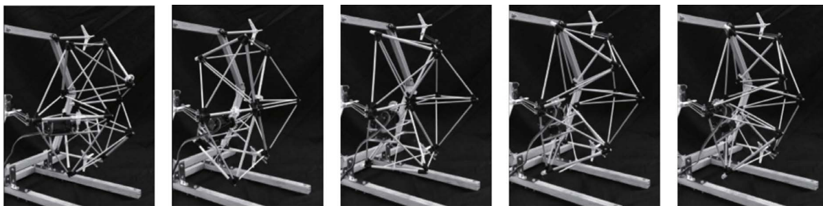
Figure 9. A thermoregulation bio-skin prototype transformed by rotation of the chameleon skin crystals
