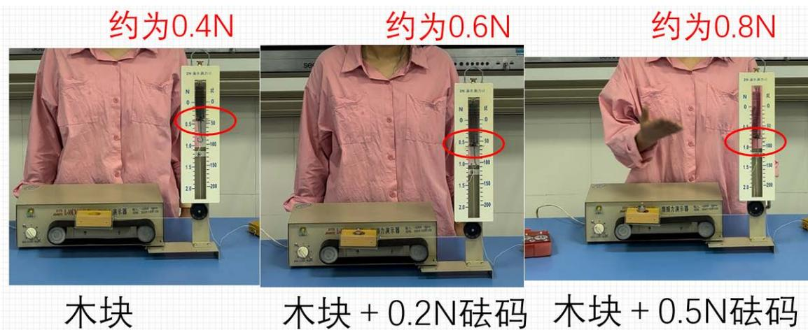
**Figure 2.** Explore the relationship between sliding friction and pressure
