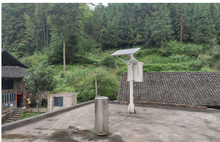
Figure 2. The rainfall station in Qiaoxi Village, Pingyong Town, Rongjiang County 图 2. 榕江县平永镇乔喜雨量站
