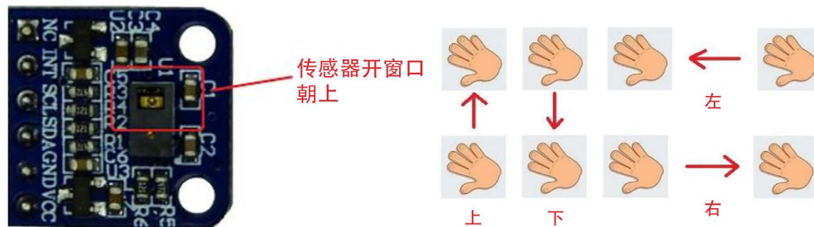
Figure 5. Gesture sensor recognizes “up, down, left and right” gestures 图 5. 手势传感器识别“上、下、左、右”手势
