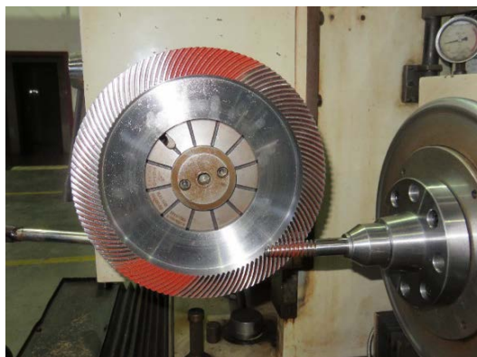
Figure 5. Super reduction hypoid gear mechanism
