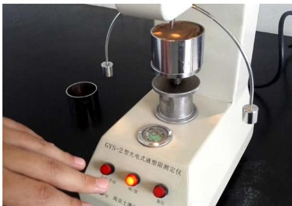
Figure 3. Liquid limit and plastic limit joint tester
