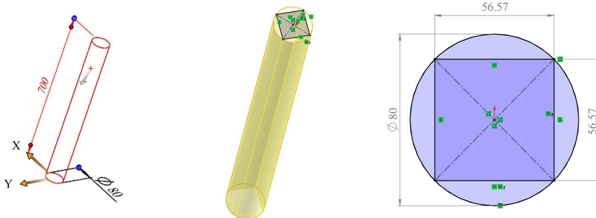
Figure 4. Design drawing of office table foot
