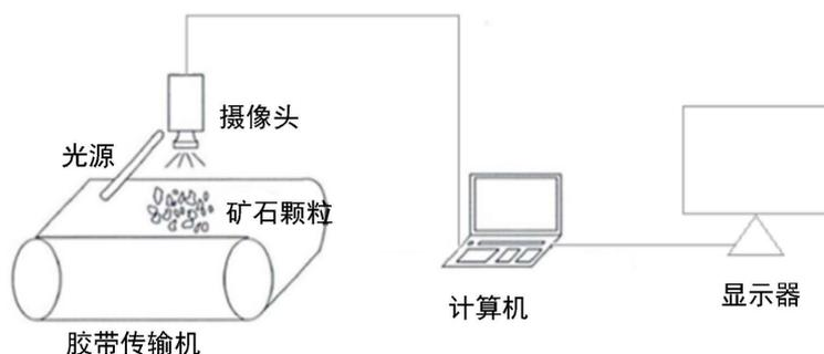
Figure 1. Detection system process
