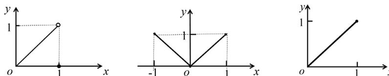
Figure 4. Any situation that does not satisfy Rolle's theorem
