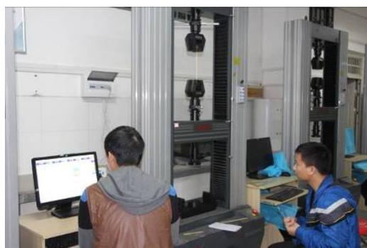
Figure 2. Bamboo specimens being loaded and data recorded by students
