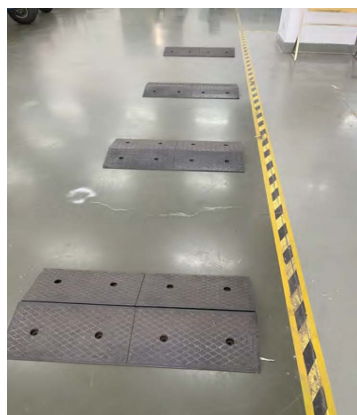
Figure 6. Half-sin belt in test 3(2)
