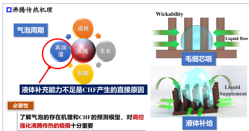
Figure 6. Mechanism of boiling heat transfer investigated based on course feedback content
