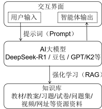
Figure 3. Diagram for constructing a DSP course teaching agent based on AI large model 图 3. 基于 AI 大模型的 DSP 课程教学智能体搭建框图
