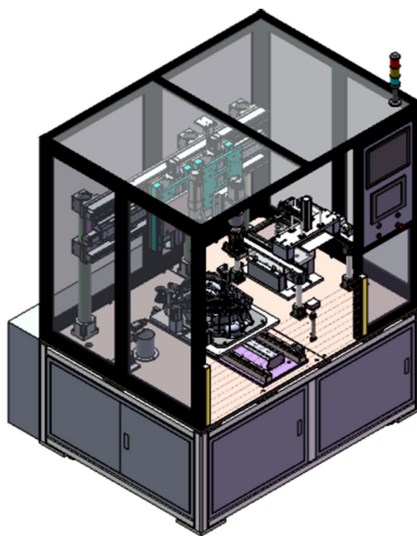
Figure 1. Lubrication, assembly and disassembly equipment for the clutch housing bearing bracket 图 1. 离合器壳体轴承支架涂油拆装设备
