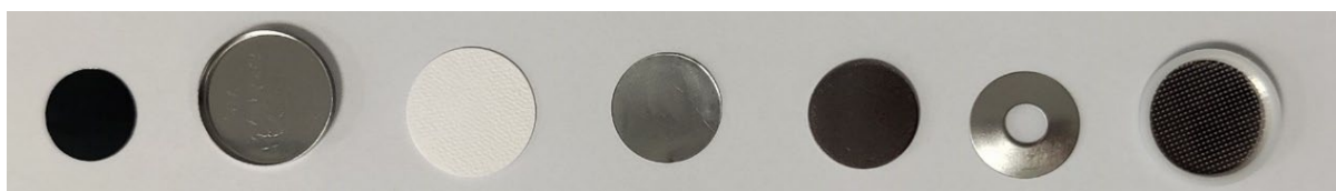
Figure 2. Components of the button battery (From left to right: positive electrode sheet, positive electrode, separator, zinc negative electrode, gasket, spring plate, negative electrode housing)
