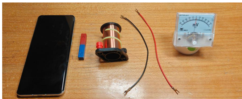
Figure 1. Experimental setup for Lenz Law based on smart phone slow-motion recording 图 1. 基于手机慢动作技术的楞次定律实验装置
