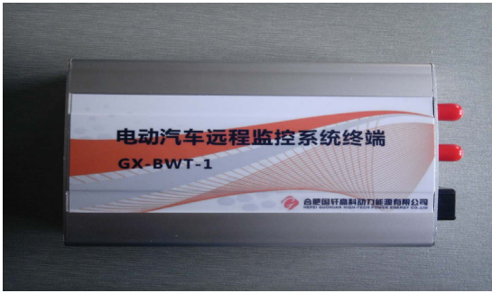
Figure 15. Implementation of the remote monitoring terminal 图 15. 远程监控的终端的实现
