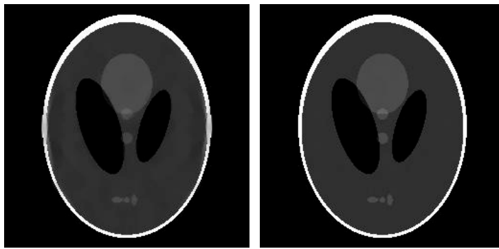
Figure 4. 14 angle reconstruction results (a) the results of the isotropic TV reconstruction algorithm; (b) the results of the anisotropic TV reconstruction algorithm
