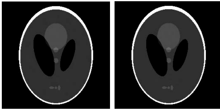
Figure 5. 16 angle reconstruction results (a) the results of the isotropic TV reconstruction algorithm; (b) the results of the anisotropic TV reconstruction algorithm
