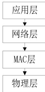
Figure 1. ZigBee reference model for communications
