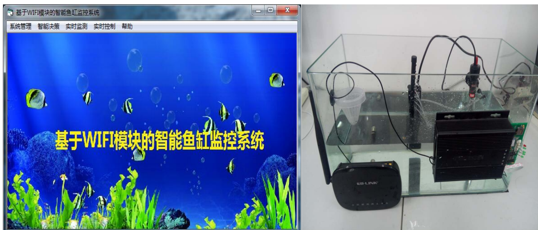
Figure 5. Application interface of remote client and physical diagram 图 5. 远程客户端应用程序界面和实物图
