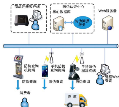
Figure 3. Traceability system diagram
