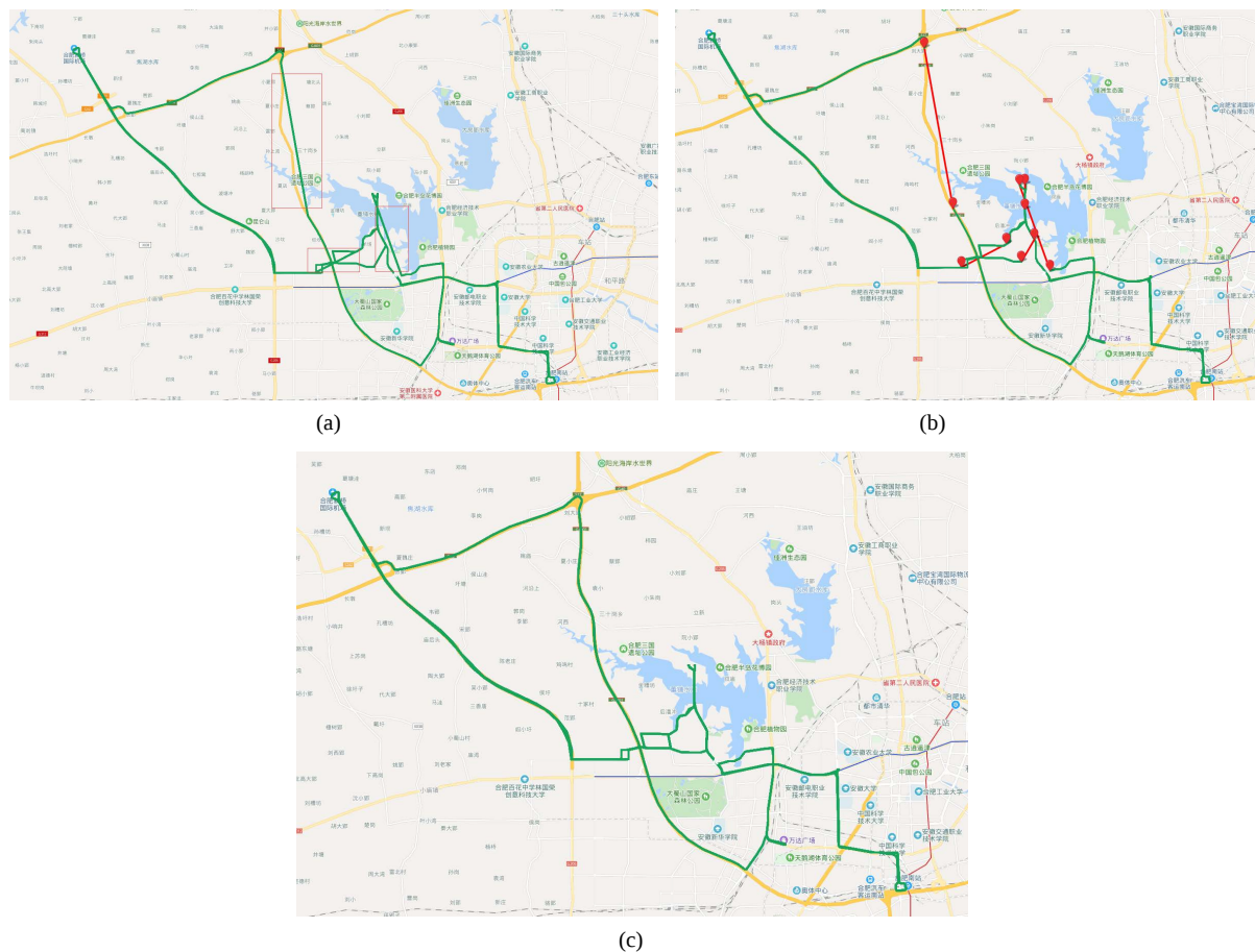
Figure 5. (a) Original trajectory (xx99E91); (b) Automatic detection and labeling of missing tracks (xx99E91); (c) Trajectory after missing trajectory compensation (xx99E91)
