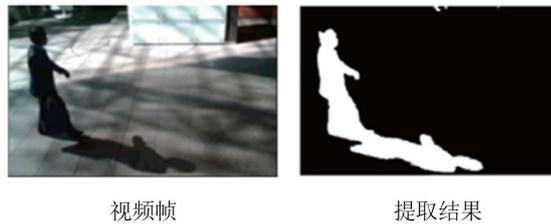
Figure 3. Moving object extraction results with shadows
