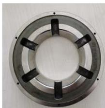
Figure 2. Standard ring gauge
