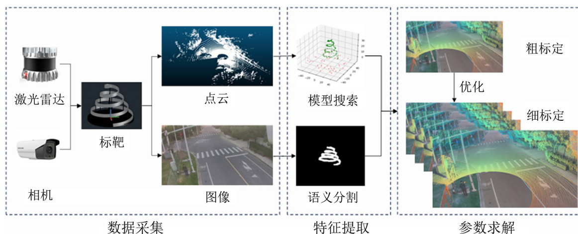
Figure 1. Architecture of the calibration algorithm
