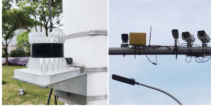
Figure 3. Installed LiDAR and camera 图 3. 激光雷达和相机
